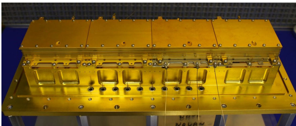
Figure 4 Gold-plated magnesium drift and field cage assembly mounted on top of the GEM-ROB assemblies inside the gas volume.
