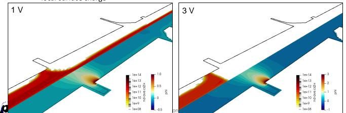
asymmetry in flow lines due to nonidentical sizes of the ambient region to satisfy meshcoupling limitations of the constant pressure source
