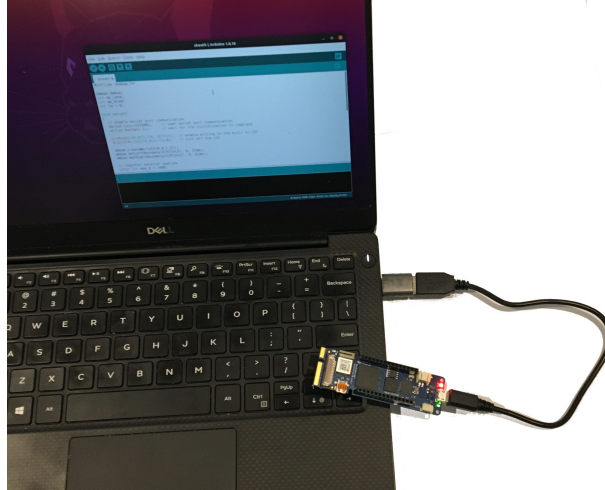
Fig. 2 Programming an Arduino is accomplished by connecting the board to a computer with a USB cable
